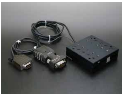
Long stroke (10mm), high resolution (5nm) piezo stage
