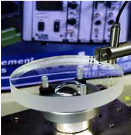
Glass surface detection sensor
